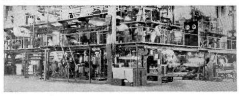
1200 Feet a Minute! That's how fast this magazine printing press gobbles up paper, At the delivery end. a sharp steel knife snaps in and out 640 times a minute to cut the paper. American Quality Springs are used to cushion the shock. They perform so well that the customer has been using them in these presses for 20 years.
